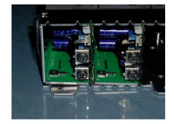
Series connection with remote sense is possible with any series combination of modules which have remote sense available.
