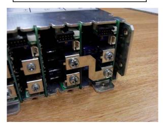
Example 4 : 2 slot E2 module with voltages combined.
