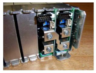
Example 3 : 1.5 slot D4 module with voltages combined.
