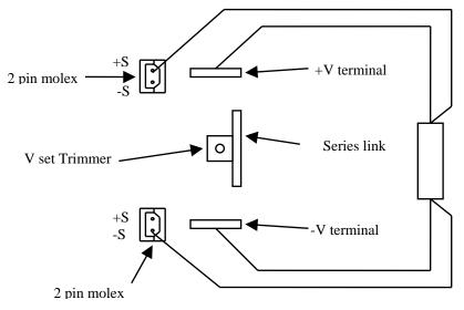
Connect +S from the top 2pin molex connector to +V of the load. Connect -S from the bottom 2pin molex connector to -V of the load.
