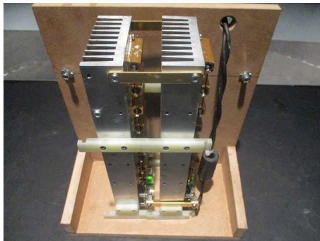
Auxiliary Equipment – Resistance load
