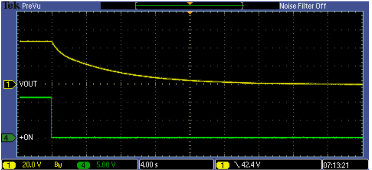
+ON: 5V/div Vout: 20V/div 4s/div Output fall with ON/OFF control(0% Load, 220Vac input)
