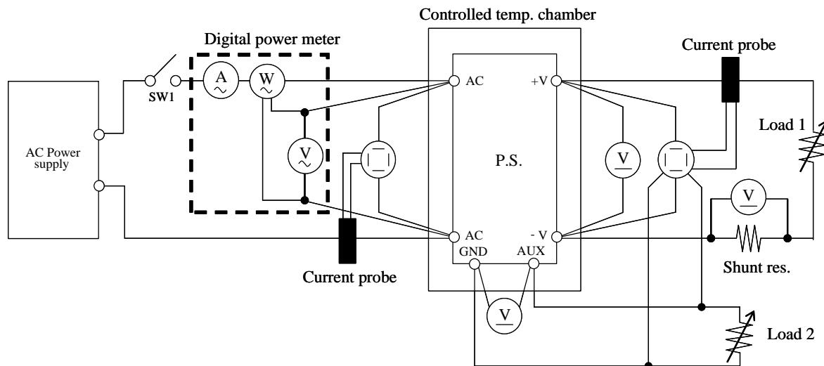
測定回路2 Circuit 2 used for determination
