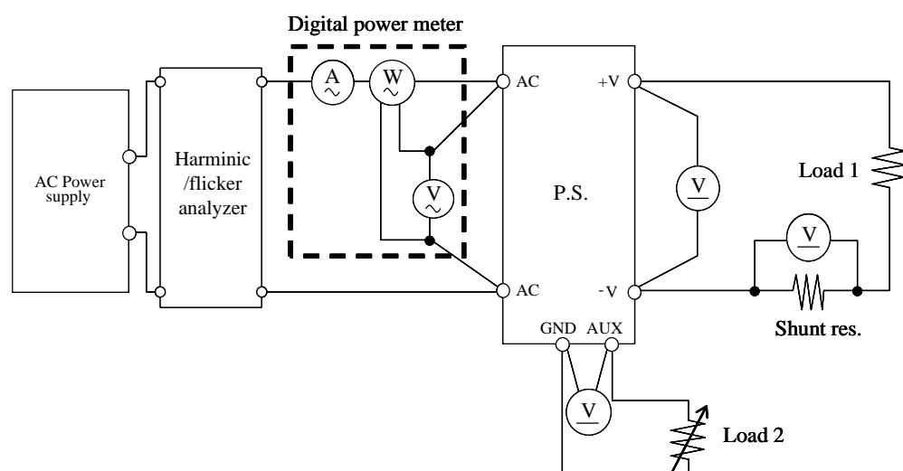
測定回路6 Circuit 6 used for determination
