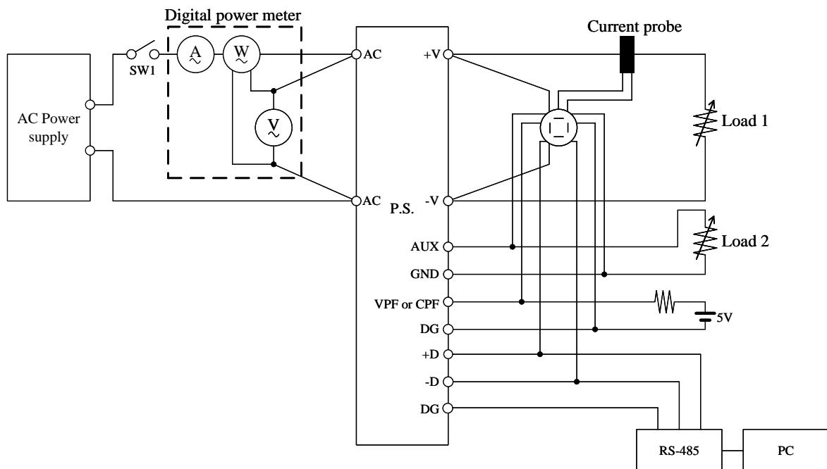
測定回路7 Circuit 7 used for determination
