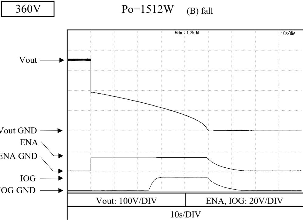
2.11 過渡応答(入力急変)特性 Dynamic line response characteristics
