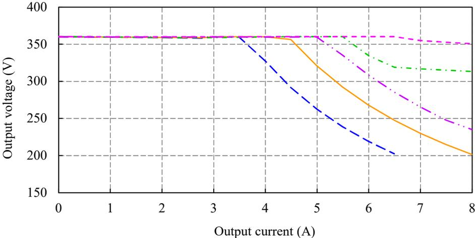
2.5 過電圧保護特性 Over voltage protection (O.V.P.) characteristics
