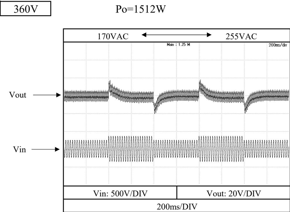
2.12 過渡応答(負荷急変)特性 Dynamic load response characteristics
