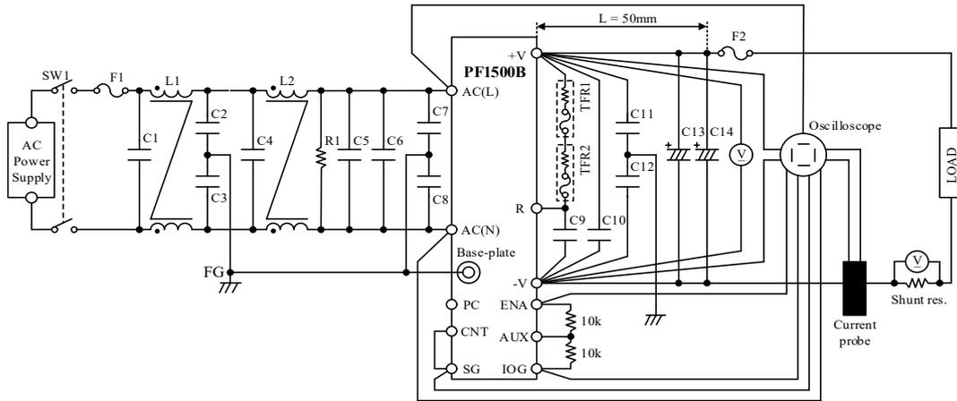
(8) 過渡応答(入力急変)特性 Dynamic line response characteristics
