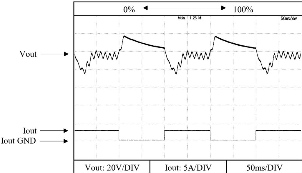
2.12 過渡応答(負荷急変)特性 Dynamic load response characteristics
