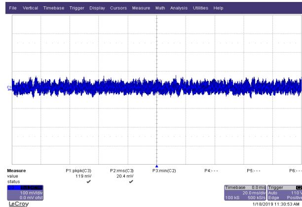
V<sub>IN</sub> = 230 VAC; I<sub>O</sub> = 10.5 A; V<sub>O</sub> = 48 VDC
