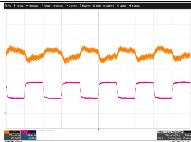
$V_{IN} = 230$  VAC; Load Step: 50% (5.25A)  $\leftrightarrow$  100% (10.5A), 1KHz
