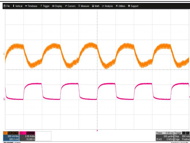
$V_{IN} = 230$  VAC; Load Step: 0% (0A)  $\leftrightarrow$  50% (5.25A), 1KHz
