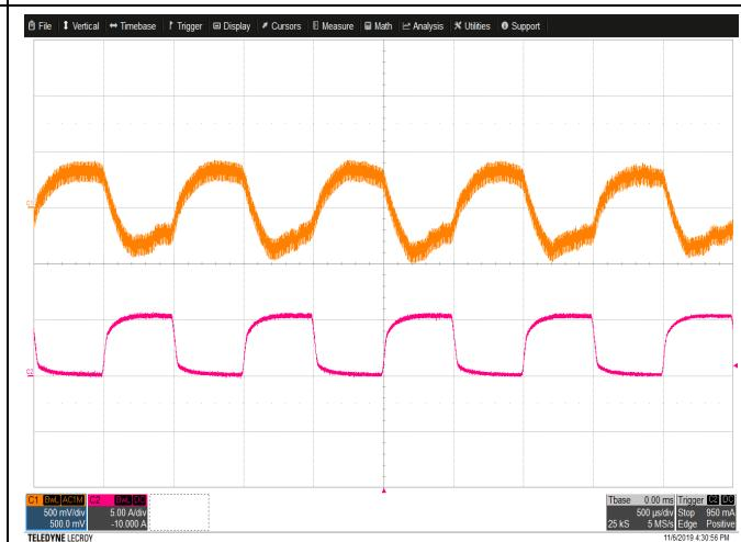
$V_{IN} = 115$  VAC; Load Step: 50% (5.25A)  $\leftrightarrow$  100% (10.5A), 1KHz
