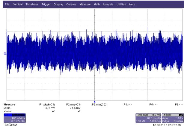
V<sub>IN</sub> = 230 VAC; I<sub>O</sub> = 1 A; V<sub>O</sub> = 48 VDC
