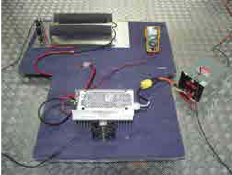
Photograph 10. RF Conducted Immunity Test Configuration
