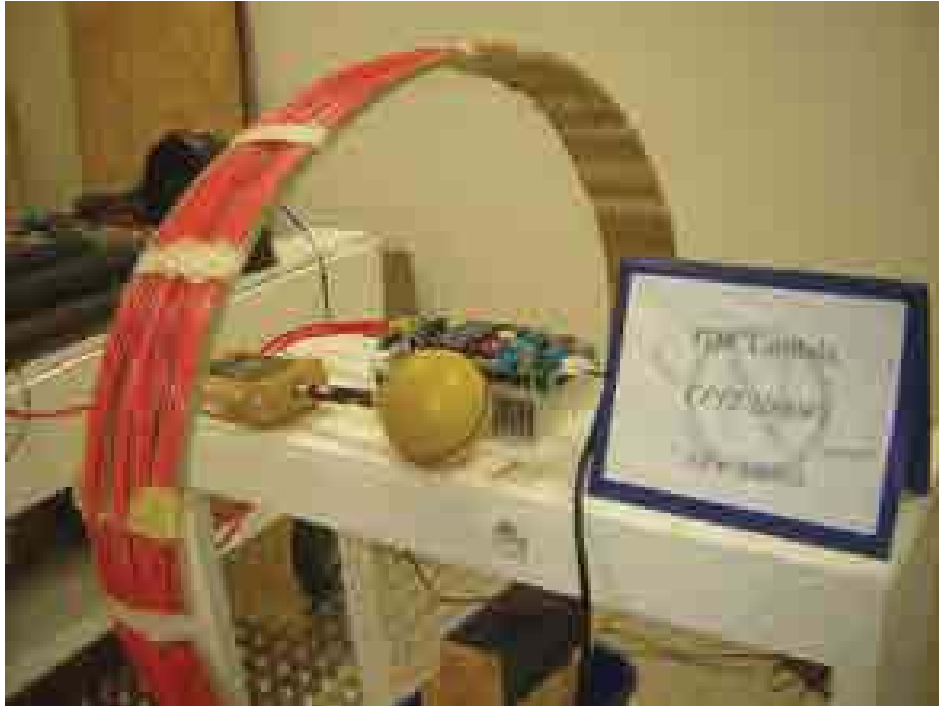
Photograph 11. Power Frequency Magnetic Field Immunity Test Configuration
