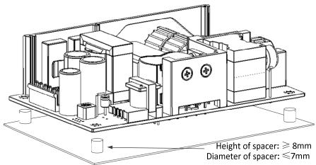
(2) Conditions to meet Isolation and Withstanding Voltage standard.
