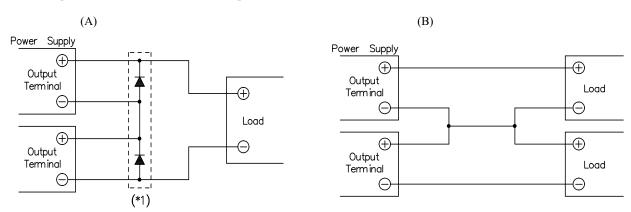
(\*1)Please select a bypass diode with maximum forward current rating more than output load current. And maximum reverse voltage must withstand each power supply output voltage.
