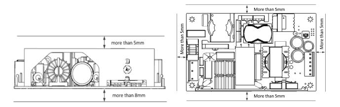
(3) (Protective Earth) should be connected to the earth terminal of the equipment. Also the mounting hole are should be connected to the Chassis by metal spacer. If not, the conducted noise, radiation noise and output noise may increase. Please refer to below setup.
