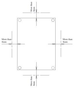
terminal (Protective Earth) must be connected to the earth terminal of the equipment, also the two mounting holes (as shown below) needed to be connected to earthed metal plane or metal chassis of end product by metal spacer to ensure EMC and EMI performance.
