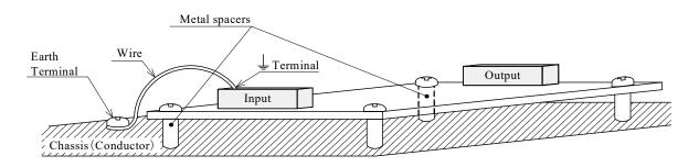
Consider the heat radiation and safety when the power supply is used in convection cooling. Please take a distance more than 15mm between the power supply and the peripheral parts. When lay out multiple units, please make sure to place 15mm or more space from each other.
