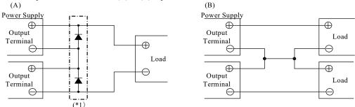
(\*1) For VS50E only in case of (A), please connect bypass diodes to prevent reverse voltage. Please select a bypass diode with maximum forward current rating more than output load current. And maximum reverse voltage must withstand each power supply output voltage.
