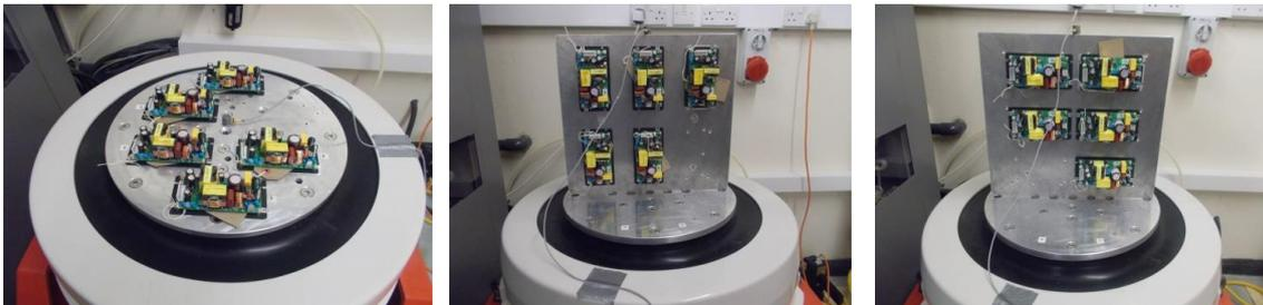
Fix the PSUT on the mounting rail with stopper on each corner.
