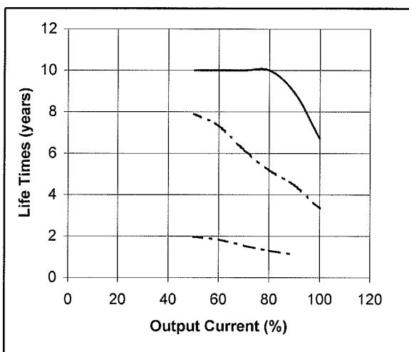
Note : E-cap life calculation is based on 24hrs/day operation.
