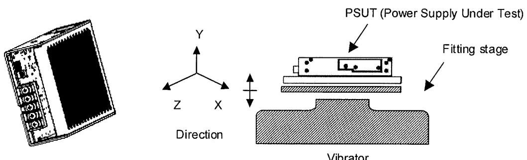
Fix the PSUT on the universal plate via two M4 tapped holes on the chassis of the power supply.
