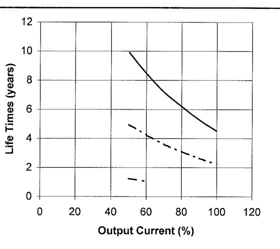
Note : E-cap life calculation is based on 24hrs/day operation.
