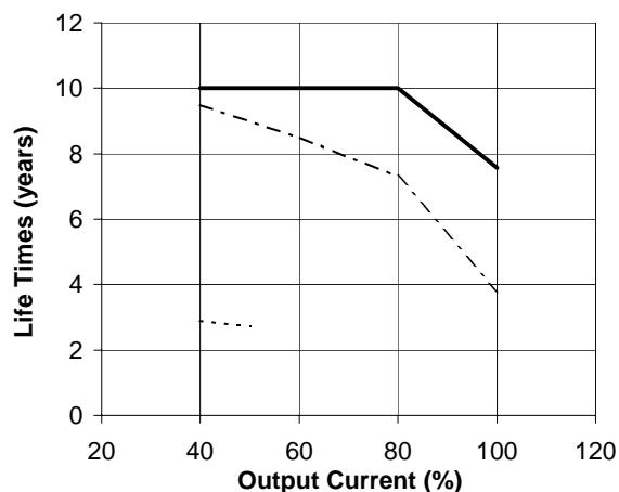
Note : E-cap life calculation is based on 24hrs/day operation.
