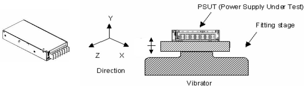
Fix the PSUT on the universal plate via two M4 tapped holes on the chassis of the power supply.
