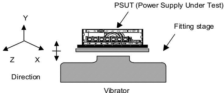
Fix the PSUT on the universal plate via two M3 tapped holes on the chassis of the power supply.
