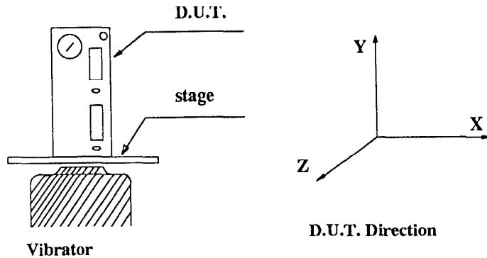
**Sweep frequency : 10 ~ 55Hz****Sweep time: 1min****Acceleration: const. (2G)****Direction: X, Y, Z.****Test time: 1H each****Result:****OK NG**
