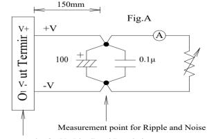
Measurement point for Vo Line/Load Regulation
