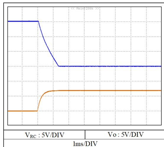
2-6. 過渡応答(負荷急変)特性 Dynamic load response characteristics
