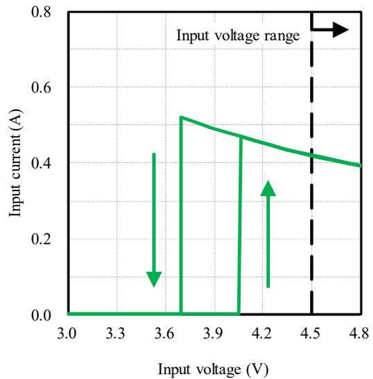
(5) 起動・遮断電圧特性 Start up and Drop out voltage characteristics
