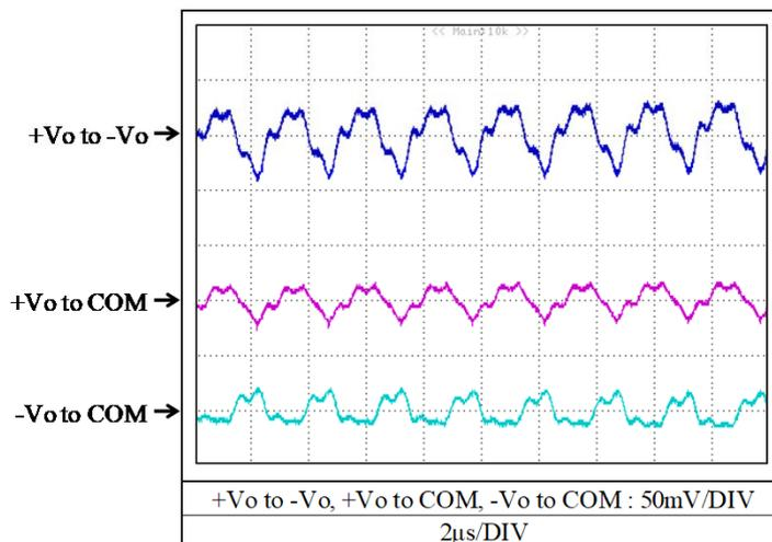
2-9. EMI特性 Electro-Magnetic Interference characteristics
