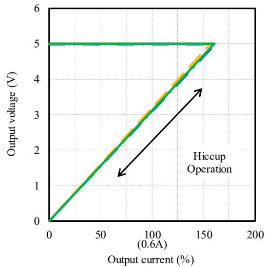
2-4. 過電流保護特性 Over current protection (OCP) characteristics
