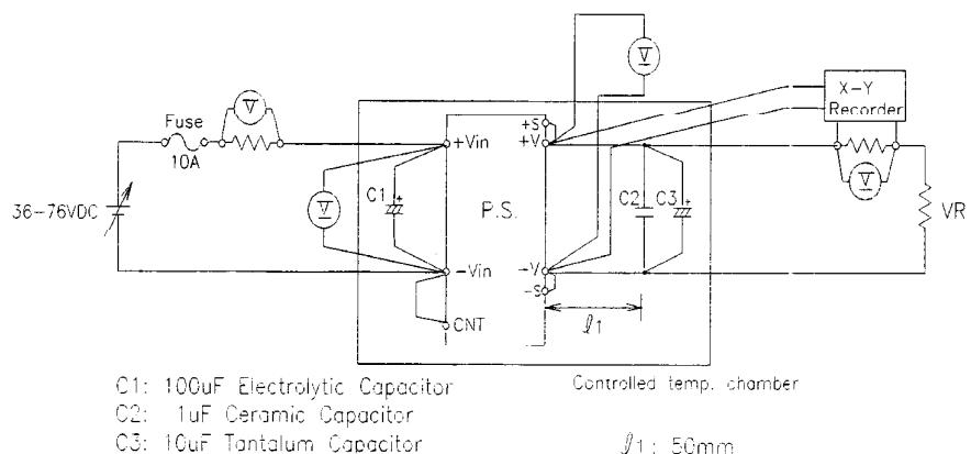
(4) 過電圧保護特性 Over voltage protection (OVP) characteristics
