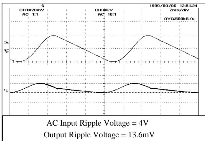
AC Input Ripple Voltage = 4V
