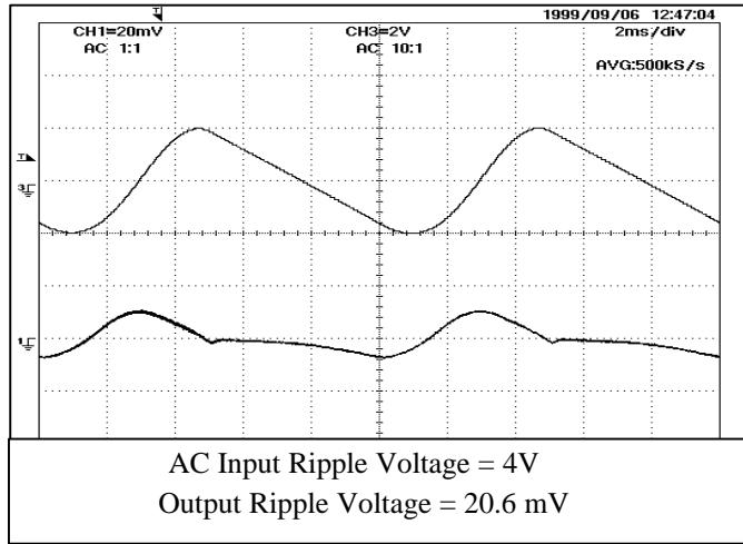
AC Input Ripple Voltage = 4V
