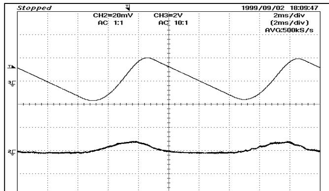
AC Input Ripple Voltage = 4V
