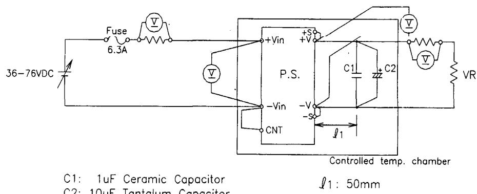
(2) 通電ドリフト Warm up voltage drift characteristics
