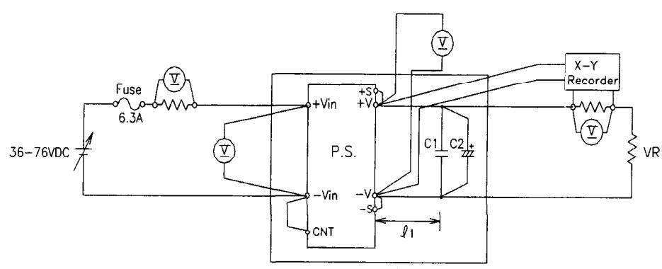
C1: 1uF Ceramic Capacitor      l1: 50mm
