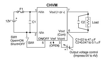
When lowering the output noise even more, keep in mind the input/output wiring, creepage and area distance, while keeping the wiring as thin as possible and layout the C2 near the Load.
