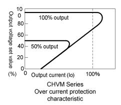
The over current protection has a hold back characteristic.
