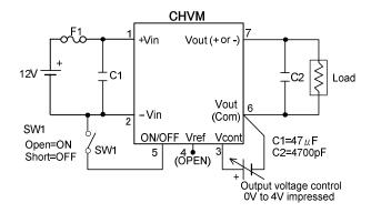
The CHVM series does not require any external parts, however when the impedance is high, for example: The distance between the power supply and converter long, the input line is thin, or the input side has a filter then connecting a capacitor C1 to the input side is recommended.
