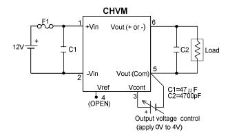
The CHVM series does not require any external parts, however when the impedance is high, for example: the distance between the power supply and converter is long, the input line is thin, or the input side has a filter then connecting a capacitor C1 to the input side is recommended.
