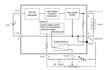
• Switching frequency (fixed) : 200kHz
