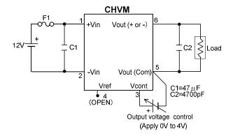
Warning 1: The ground line (2pin, 5pin) between the input/output, and the case are internally connected. Warning 2: Vref is  $4V \pm 0.3V$  (When external  $VR=5K\Omega$ )
