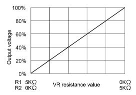
Output voltage—Output control voltage characteristic
