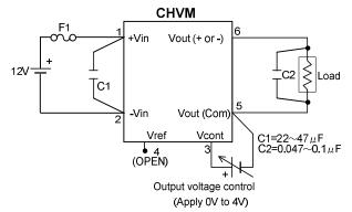
When lowering the output noise, the wiring of the input and output should be as short as possible. Place C2 closest to the load, paying attention to creepage and clearance distances.
