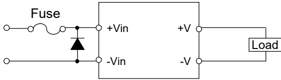
Fig.1-5 Protection for Reversed Connection of Input
