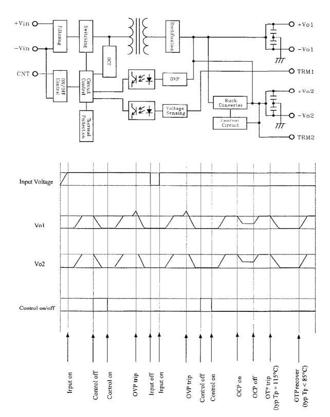
Note: This timing diagram is for Negative Logic "ON/OFF Option.
