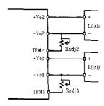
The equations and graphs for the required external resistor ( $R_{adj}$ ) value to obtain a percentage output voltage change of  $\Delta Vo\%$  is as shown in the next page.
