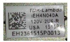
Note: The above markings are the minimum requirements required by the safety lab. For the final production samples, the additional markings which do not give rise to misunderstanding may be added.
