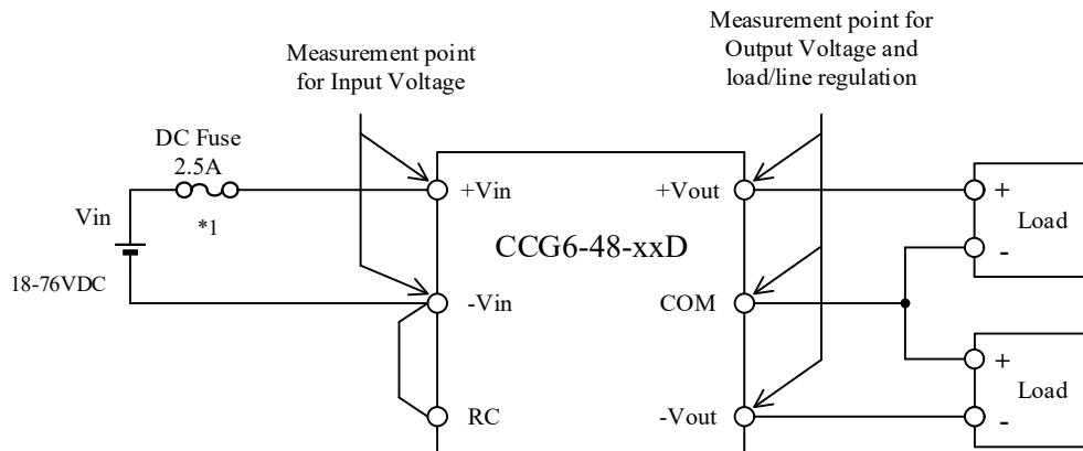
\*Read instruction manual carefully, before using the power supply unit.
