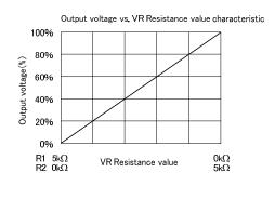
In the output voltage vs. VR resistance value characteristic graph, the resistance values of R1 and R2 are reference values. When setting the output voltage to a fixed output with a fixed resistor, first decide R1 and R2 with the variable resistor. Use a variable resistor with good temperature characteristics.
