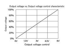
Do not apply more than 6V + 3% to the voltage applied to Vcont.
