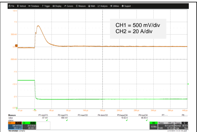
Vo = 3.3V Typical output voltage transient response to load step from 75% to 25% of full load with output current slew rate of 1A/μs, Cext = 330 μF capacitor.
