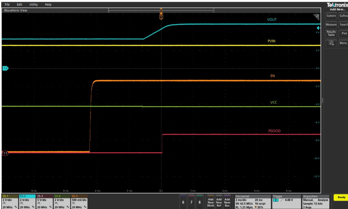
Figure 7 Startup into pre-bias. Max 70% of Vout. (Ch1:PV IN , Ch2: V OUT , Ch3: PG, Ch4:V CC , Ch5: Enable)
