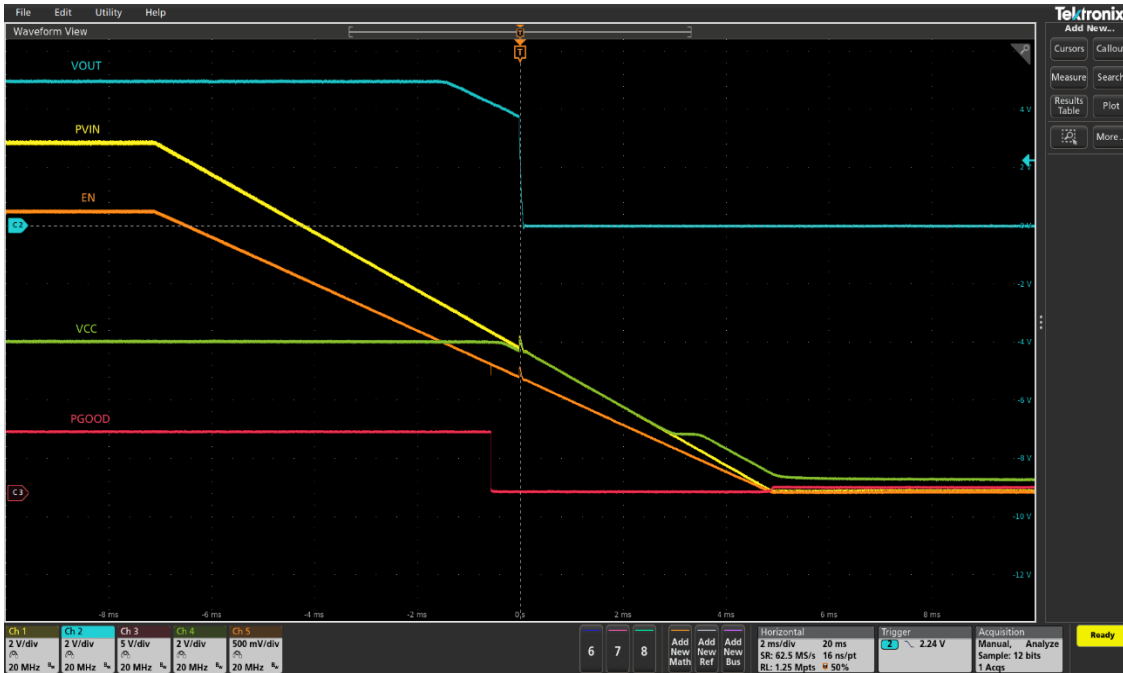
Figure 5 Shutdown with Enable de-assertion at 3A load (Ch1:PV IN , Ch2: V OUT , Ch3: PG, Ch4:V CC , Ch5: Enable)
