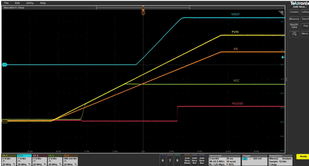
Figure 3 Startup with no load (Ch1 : PV_{IN} , Ch2: V_{OUT} , Ch3: PG, Ch4: V_{CC} , Ch5: Enable)
