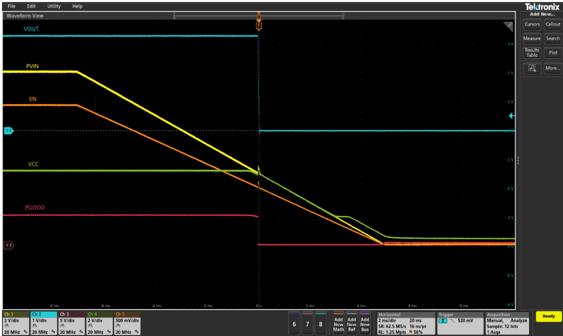
Figure 5 Shutdown with Enable de-assertion at 4A load (Ch1:PV IN , Ch2: V OUT , Ch3: PG, Ch4:V CC , Ch5: Enable)
