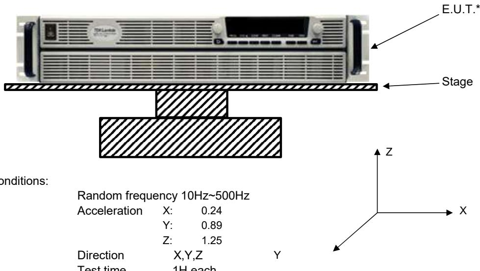
\*E.U.T. is fixed to vibrator surface by mounting straps
