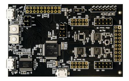
The development kit comes with necessary software including InvenSense MotionLink, a GUI based development tool and embedded Motion Drivers for ICP-10125.
